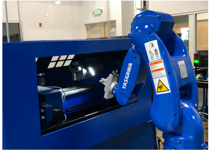
MACHINING STATION: Industrial robot arm serving components into a CNC machine
